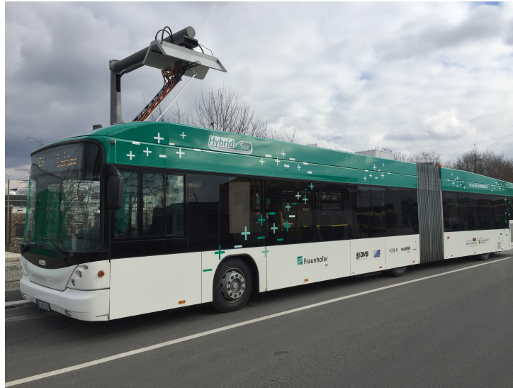
Figure 1: The city bus which was modified and evaluated during the SaxHybrid PLUS project in 2014 during a recharge operation
